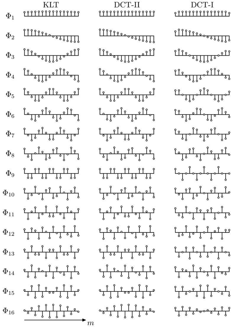
Figure 1: KLT, DCT-I and DCT-II basis functions with  $N = 16$ ,  $\rho = 0.95$ .
